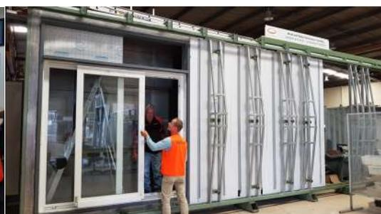
Photos of testing and certifying YZY windows in laboratory, Australia
